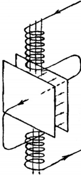
Figure 2: Schematic diagram of a "flux" capacitor.
