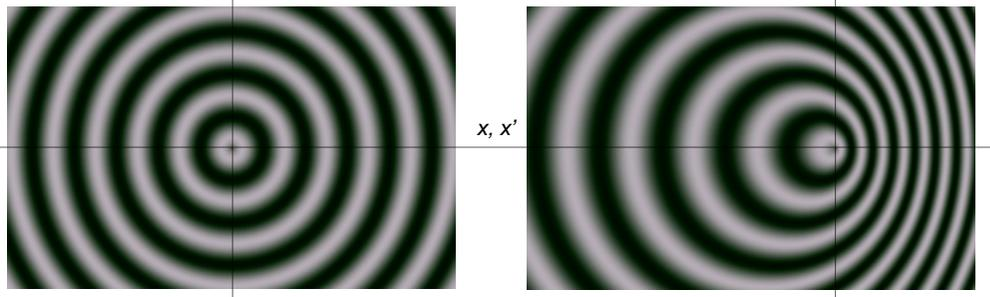
Fig.1 shows a wave source at rest ( $v=0$ ) in the medium (the electromagnetic ether). Fig.2 shows another source that moves at a constant speed ( $v>0$ ).
