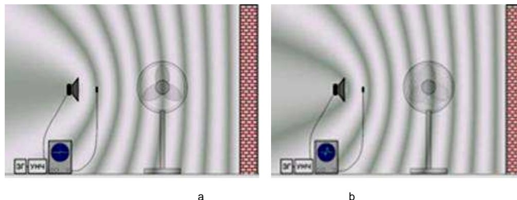
Figure 1 The appearance of the air flow between the speaker and the wall (a thread is created fan) leads to deformation of the interference pattern and the displacement of the control node in the direction of the wall. Package of standing waves is compressed.
