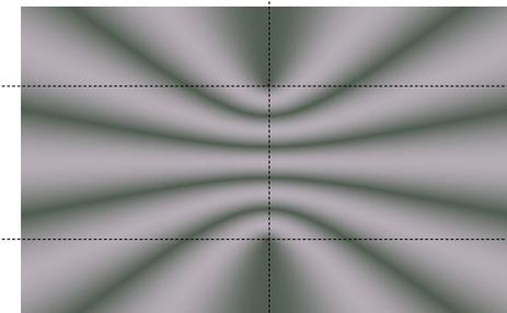
Speed of systems increases. The distance between the sources is constant. Standing waves and interference field is compacted (compacted).
