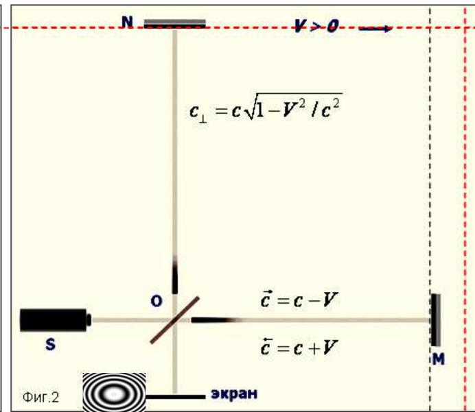
Rays come to the screen at same time. The phase shift is absent. In the center of the screen a bright spot
