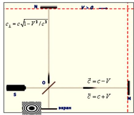
Fig.1 Rays come to the screen at different time. In the center of the screen is a dark spot.
