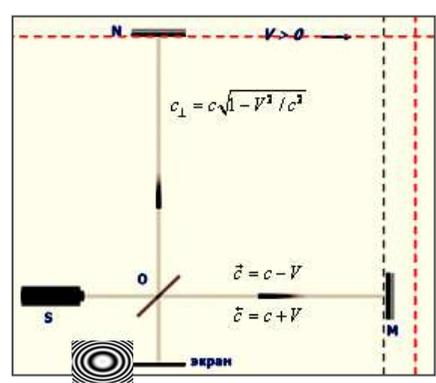
Fig.1 Rays come to the screen at same time. In the center of the screen is a bright spot.
