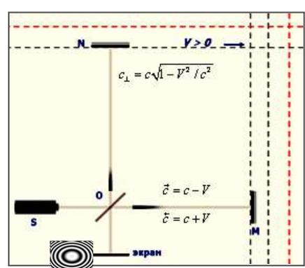
Fig.2 Rays come to the screen at same time. In the center of the screen is a bright spot.
