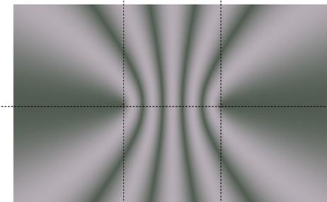
The distance and the phase shift between the wave sources are unchanged. Increasing the speed of the system leads to compression of standing waves and the compaction of the interference field.
