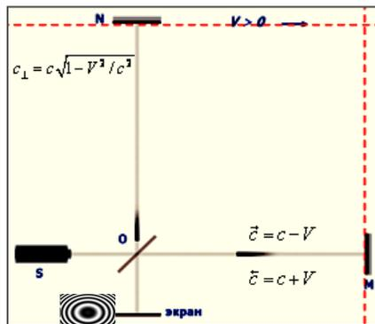
Fig.2 Rays come to the screen out of phase. In the center of the screen will be a dark spot.
