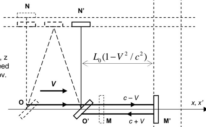
Dimensions in x, y, z depend on the speed of the rule of Ivanov.
