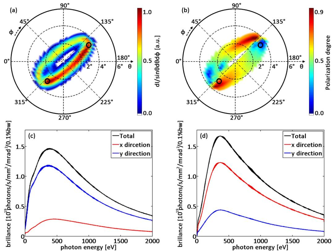
**Figure 3. Intensity and polarization distributions of X-ray radiation.** (a) Far field radiation intensity distribution, (b) polarization distribution, (c) radiation spectrum of the marked upper right point and lower left point (d).
