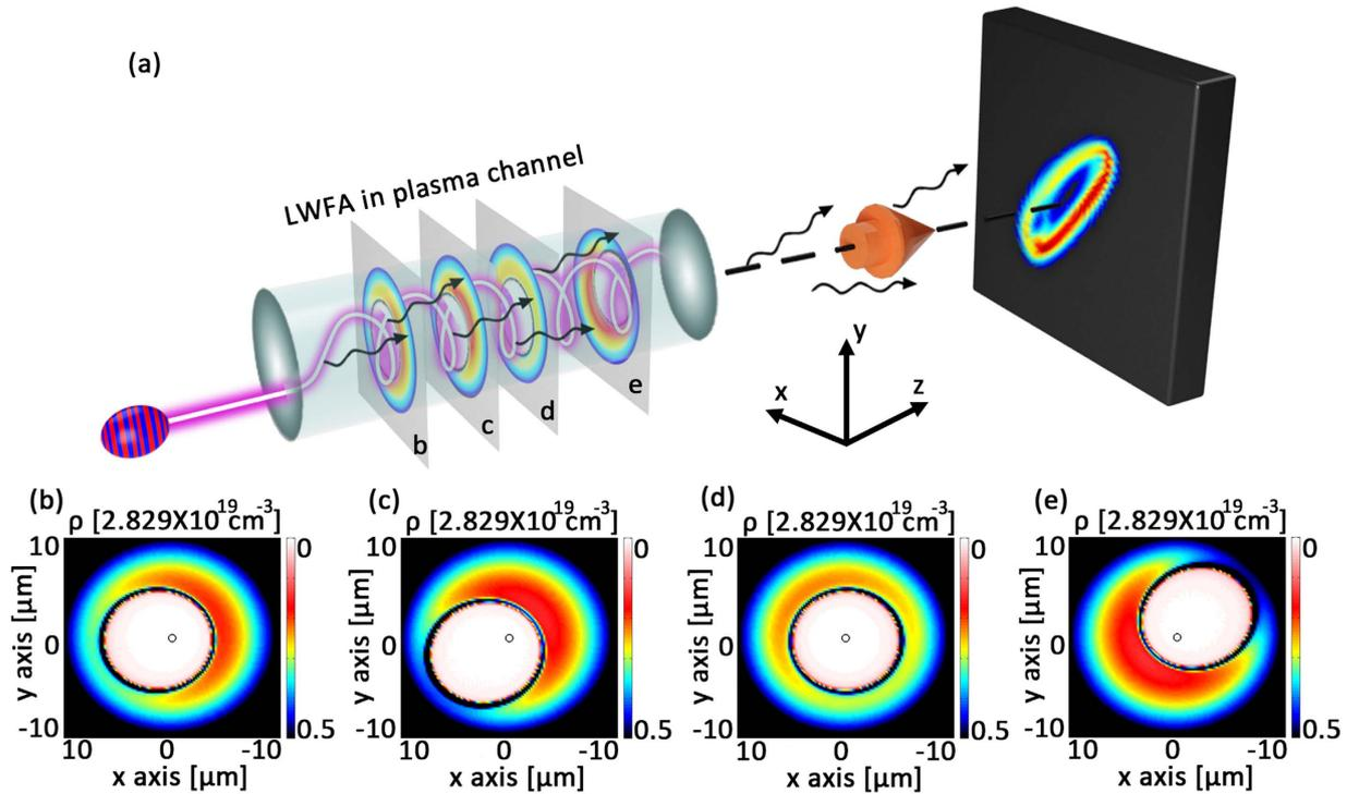
**Figure 1.** Sketch of the radiation source from a helical plasma undulator based on LWFA. (a) Spiral motion of laser pulse, wakefield in the plasma channel and the far field X-ray radiation distribution. (b–e) are the electron density distributions of the transverse slices of the accelerating bubble structure with largest radius at  $t = 133$  fs (b),  $t = 600$  fs (c),  $t = 1200$  fs (d),  $t = 1800$  fs (e).
