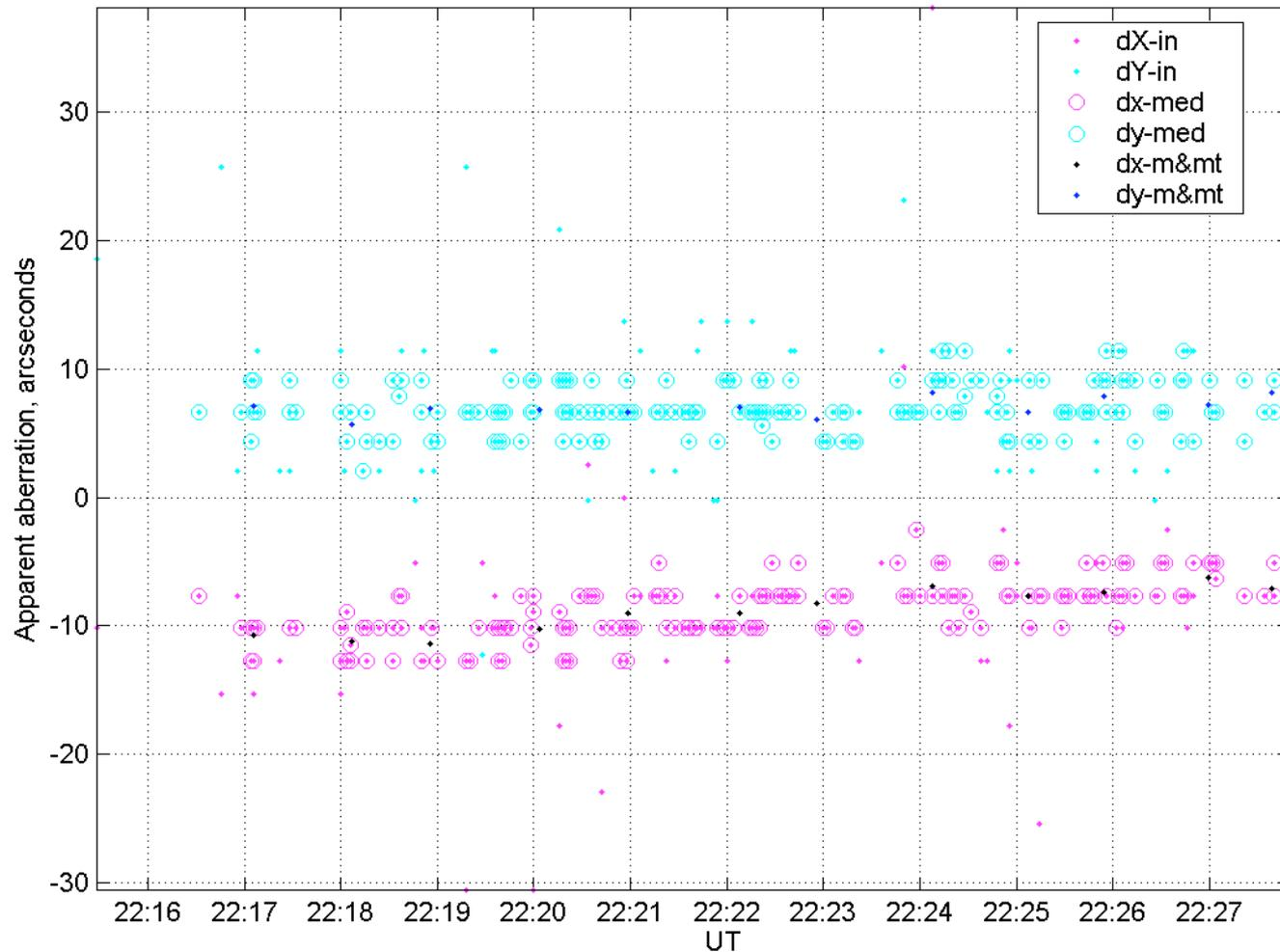
Satellite LAGEOS-1 28.07.2007. Distribution in the field of view of the telescope of measured deviations of the image of the satellite from direction of the laser beam emission (x is for abscissa, y is for ordinate): raw (dX-in, dY-in; each couple of points correspond to one frame), after median filtering (dx-med, dy-med), after use of sliding average filter to median filtered data (dx-m&mt, dy-m&mt).
