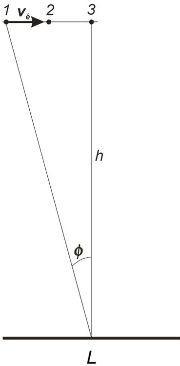
1.3 – Sequence of satellite positions; L – laser ranging station;  $h$  – distance between station and satellite;  $\phi$  – angle of velocity aberration.
